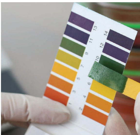
Figure 12 : pH test strips (litmus paper) are used for simple on-site estimation of pH levels in a water body.
